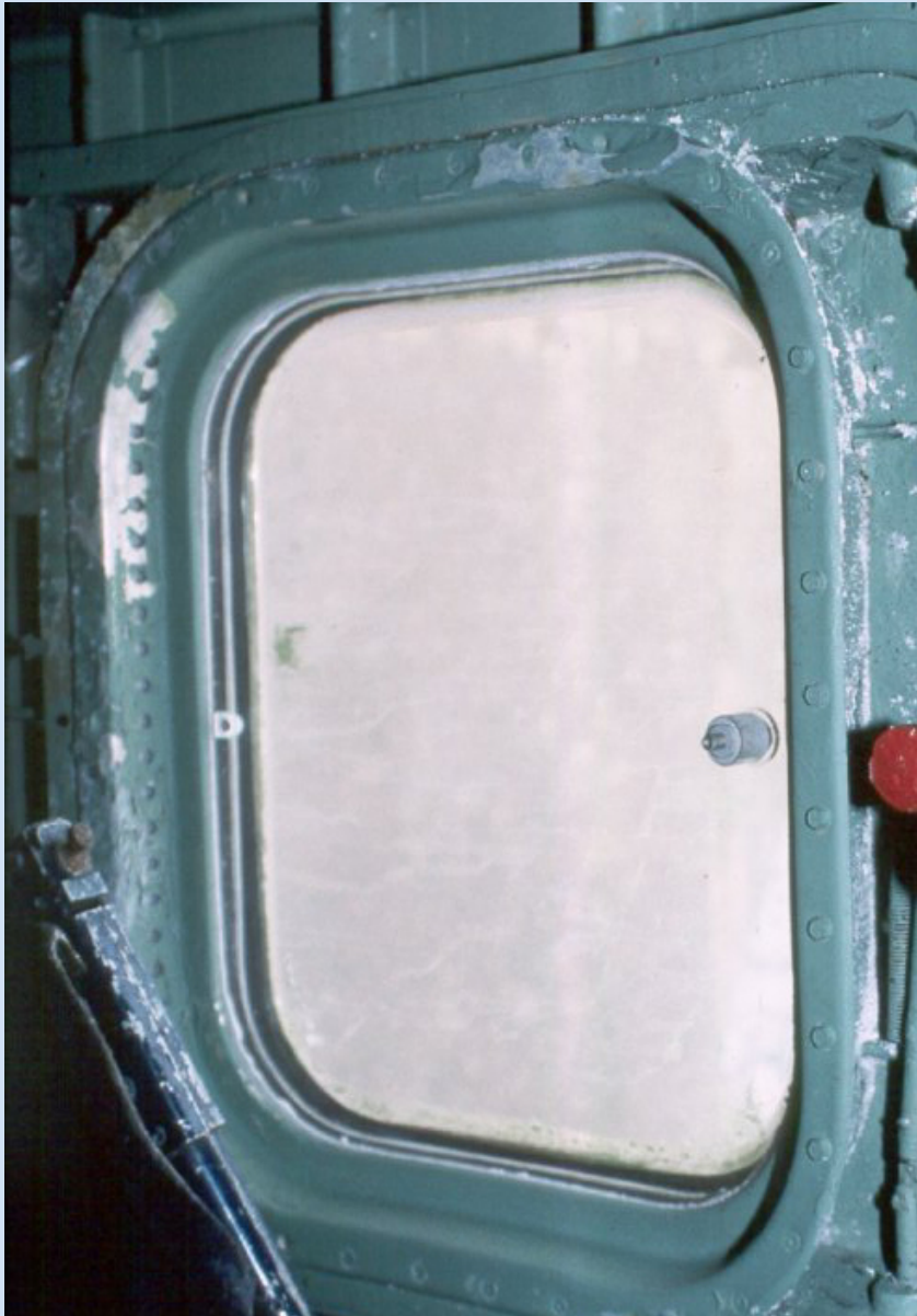
On closer inspection, the Comet airplane windows propagated cracks despite being rounded with a quarter circle fillet.
